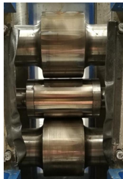
Figure 1. BFI's 3 roller testing equipment.
