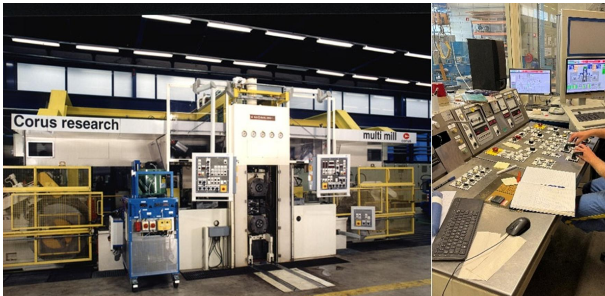
Figure 2. Semi-industrial cold rolling mill of Tata Steel Ijmuiden.
